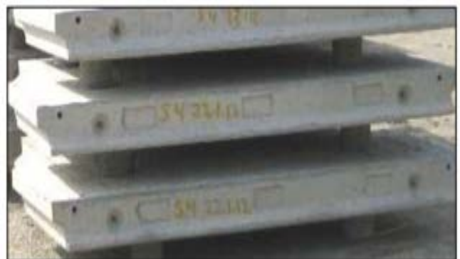
Panel type and date of casting painted on EPDM location.
